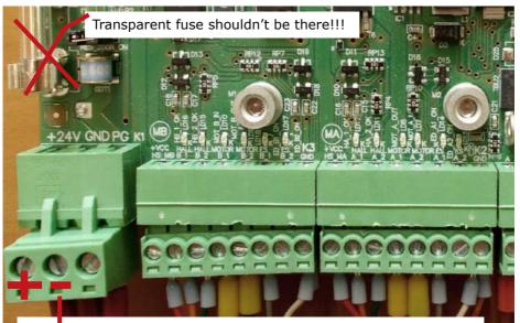
Before you connect power system be aware of plus and minus in a right terminal. Connect one wire into the plus and the other one into the minus!
